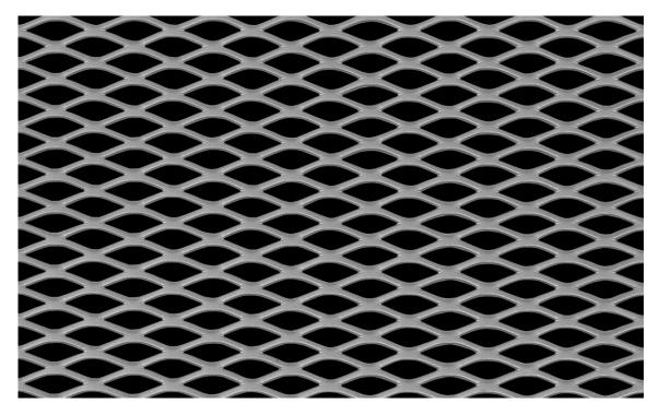
LW Pitch:19.05mmStrand Width:2.00mmSW Pitch:8.00mmThickness:1.20mmWeight:4.71 kg / m2Open Area:50%
